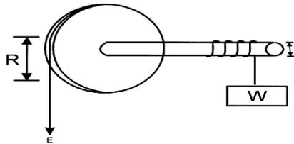
i) Show that the velocity ratio (V.R) of this machine is given by  $\frac{R}{r}$
