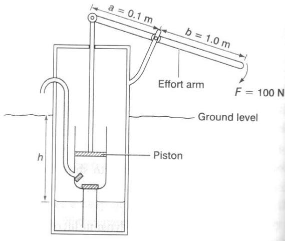
Take  $a=0.1\text{m}$ ,  $b=1.0\text{m}$ ,  $F=100\text{ N}$ , the diameter of the piston =  $5\text{cm}$ ,  $g=10\text{ N kg}^{-1}$  and the density of water =  $1.0 \times 10^3\text{ kg m}^{-3}$ .
