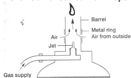
(i) Explain how the air is drawn into the barrel when the gas supply is opened.
